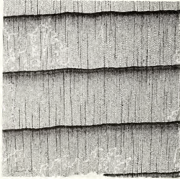
FIGURE 2-30.—Western redcedar. Cross section magnified 15 diameters.
